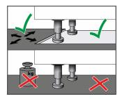
As wood is a natural material, the floor works and moves. The floating installation and expansion gap of minimum of 10 mm at perimeter and at other vertical obstacles ensure enough leeway for it to flex and expand slightly.
